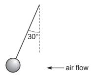
The ball is suspended by a light string and weighs 0.15 N.
