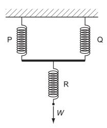
Springs P and Q are identical and have spring constant k. Spring R has spring constant 3k.
