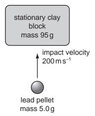
The pellet hits the block with an initial velocity of  $200\,\mathrm{m\,s^{-1}}$ . It embeds itself in the block and does not emerge.
