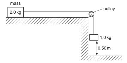
What is the speed of the  $2.0\,\mathrm{kg}$  mass as the  $1.0\,\mathrm{kg}$  mass hits the floor, having fallen a distance of  $0.50\,\mathrm{m}$ ?
